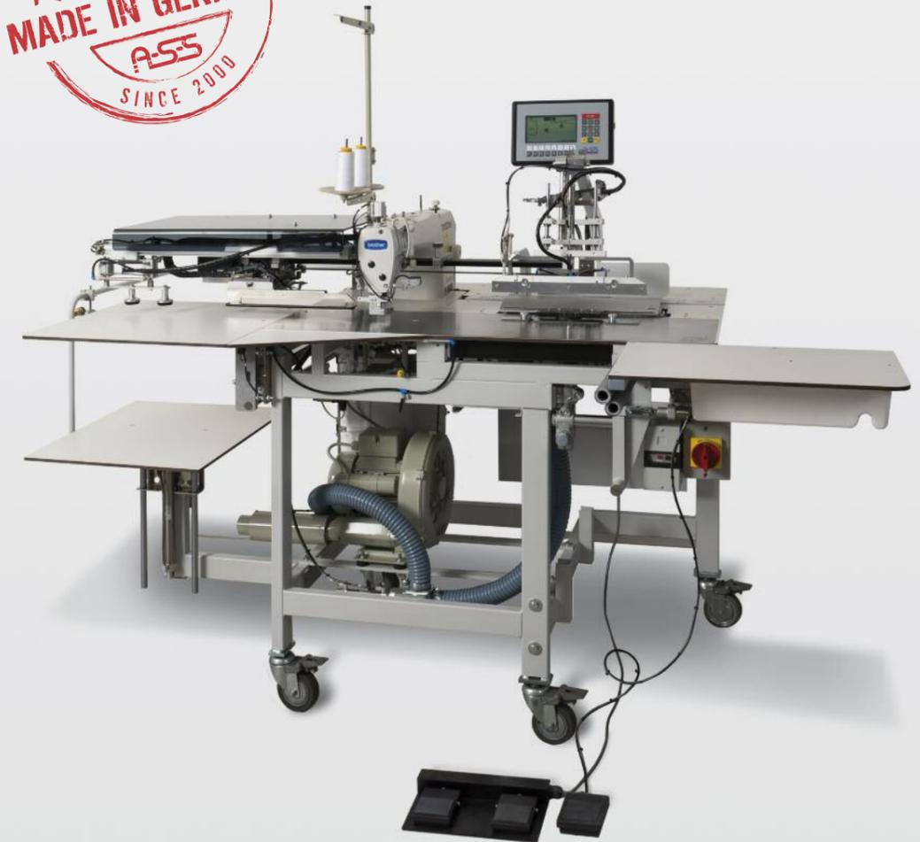
The BASS 5310 is a sewing system for processing straight and curved side seam pockets pockets as well as all straight pocket facings on pocket pouches of the front and rear sides of trousers.
