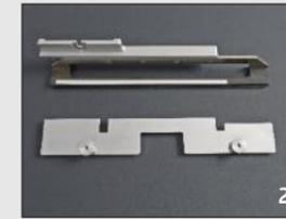
Set-up changed for straight pockets in the side seam (Figure 2)
