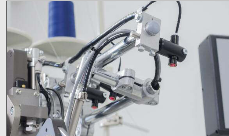
Laser markings for accurate and clear positioning
