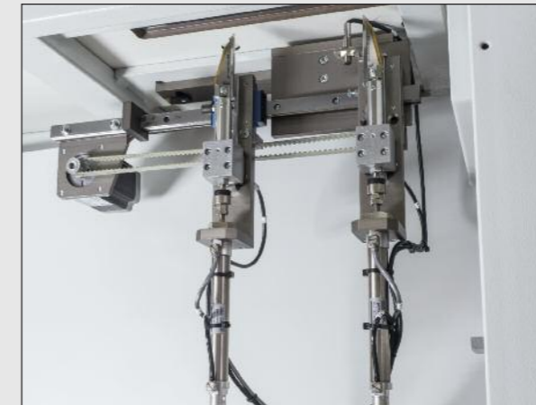
Cutter block with stepper motor drive
