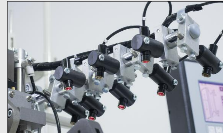
Accurate positioning by eight position lamps
