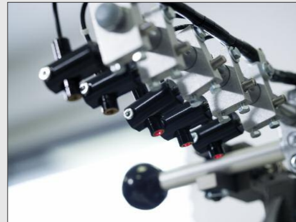
Laser markings indicate the exact pocket pouch position
