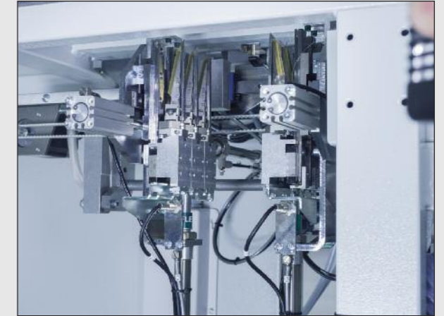
Cutter block for straight and slanted corner cuts
