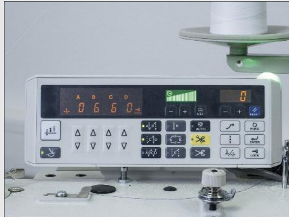
Control panel for adjusting various sewing functions
