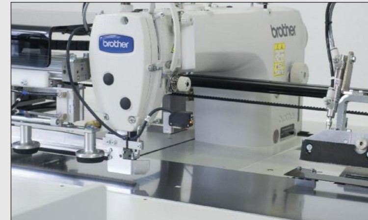
Seam length detection by the photo cell
