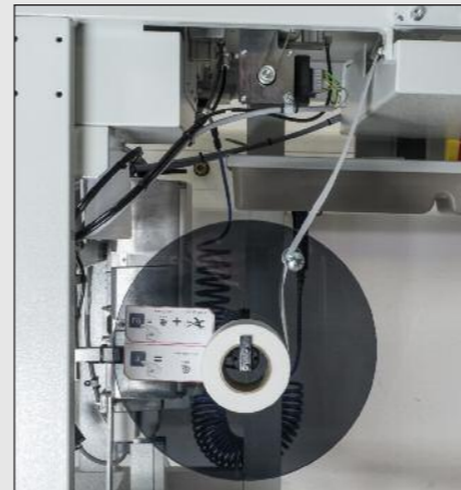
Stepper motor-controlled fleece feed
