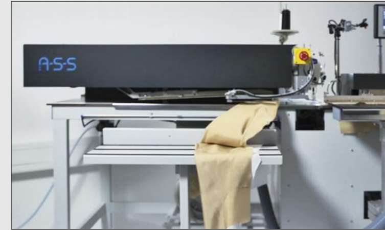
Automatic de-stacking of the sewed parts
