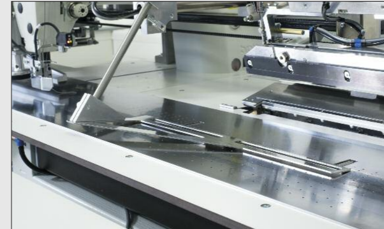
Retracted ruler for placing the zipper and fly piece
