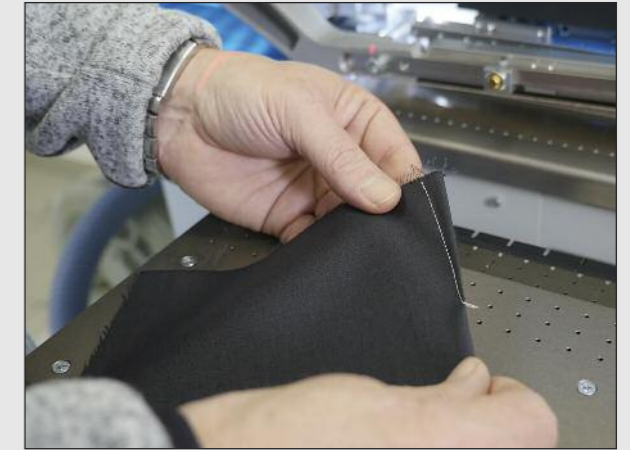
Accurate stitching on the dart tip (no cone formation)
