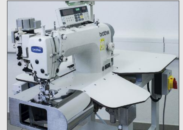
Working table shaped for ease of production
