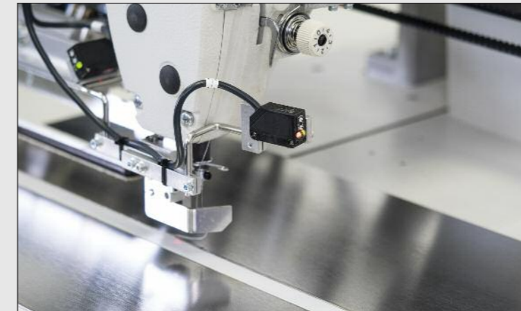
Photocells for detecting the start and end of the seam
