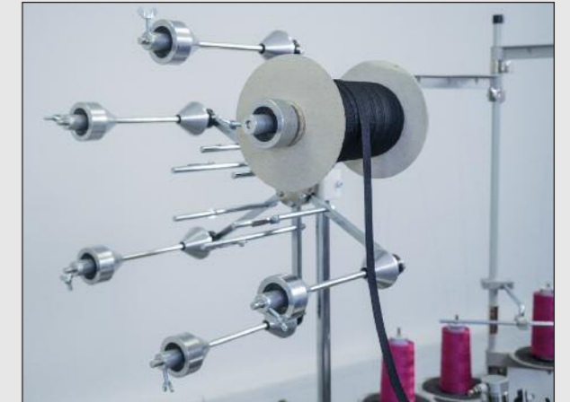
Bobbin holder and magazine function
