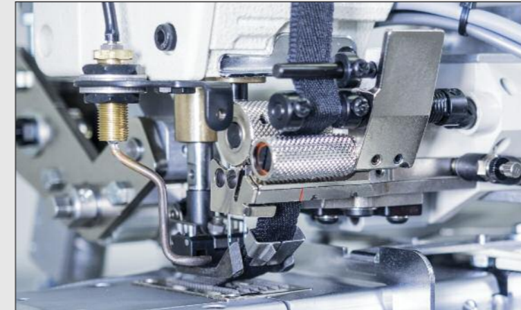
Exact tape guide to the sewing base
