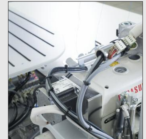
Stepper motor-controlled differential and top transport
