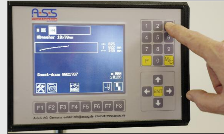
Acceptance and sewing the programmed darting machine with the X-Y controller
