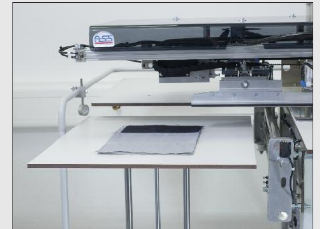
The stacker places the sewing parts for the subsequent operation
