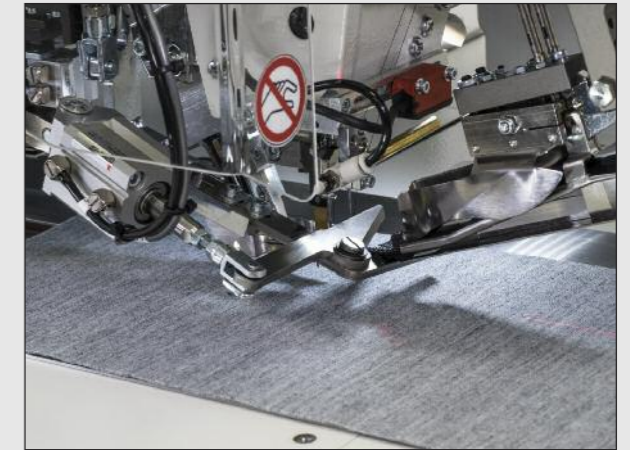
Pneumatic scissors for cutting off the endless zipper
