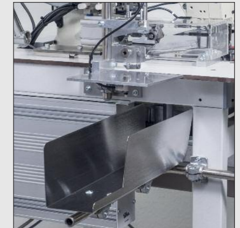
Automatic removal and de-stacking (optional)
