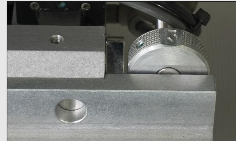
Adjustment of the stitching width using an adjusting wheel
