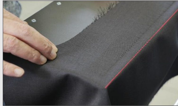
Placing the sewing part on the marking lights of the pre laying station. Fixing it with a vacuum
